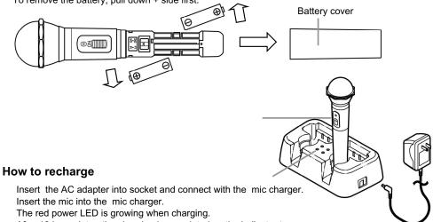
After 10 hours later, the charging is completed as the indicator turns green.
