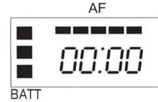
The LCD segments on the left show the approximate remaining battery life (from 1 to 3 segments) with 3 segments meaning maximum battery power. The bottom segment will blink when the battery power falls to less than 2.2V and indicates that it is time to replace the batteries. Azden recommends the use of Alkaline batteries only.
