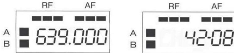
Using either the UP or DOWN button [s] the desired receiving frequency or channel number can be set. Tapping the button steps through the frequency or channel number one at a time while pressing and holding the button moves through the frequencies or channel numbers rapidly. There are 188 different frequencies or channel numbers to choose from. Once the desired frequency or channel has been determined be certain to set both the transmitter and the receiver to match.
