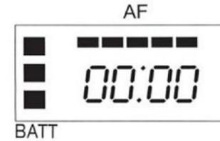
The LCD segments on the left show the approximate remaining battery life (from 1 to 3 segments) with 3 segments meaning maximum battery power. The bottom segment will blink when the battery power falls to less than 2.2VDC and indicates that it is time to replace the batteries. Azden recommends the use of Alkaline batteries only.
