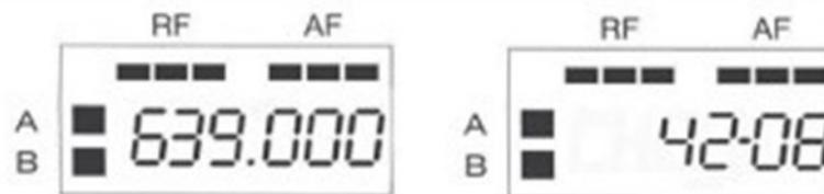
Using either the UP or DOWN button [o] the desired receiving frequency or channel number can be set. Tapping the button steps through the frequency or channel number one at a time while pressing and holding the button in moves through the frequencies or channel numbers rapidly. There are 188 different frequencies or channel numbers to choose from. Once the desired frequency or channel number has been determined, be certain to set both the transmitter and the receiver to match.
